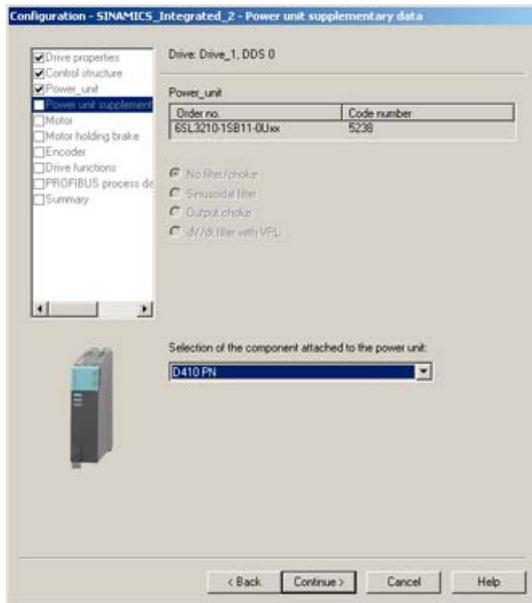
Figure 4-4 Selecting an adapter module
