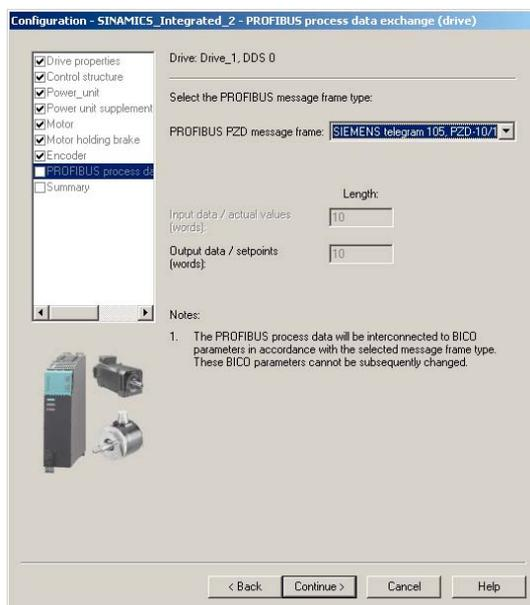
Figure 4-8 Selecting the PROFIBUS message frame
