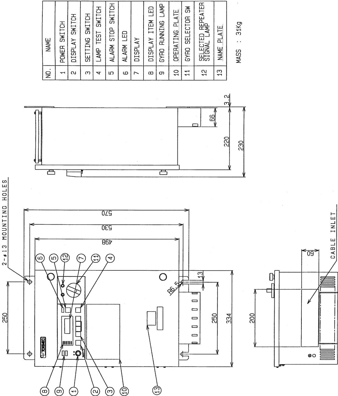
Figure 5-9 Change Over Unit (Bulkhead Type) Outline
