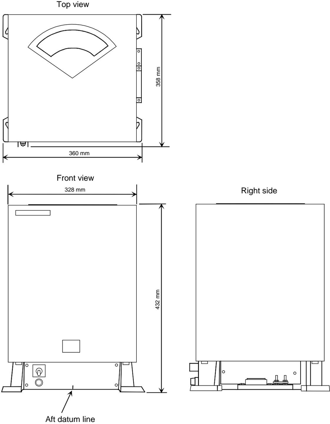
**Figure 4-1 Master Compass Dimensions**
