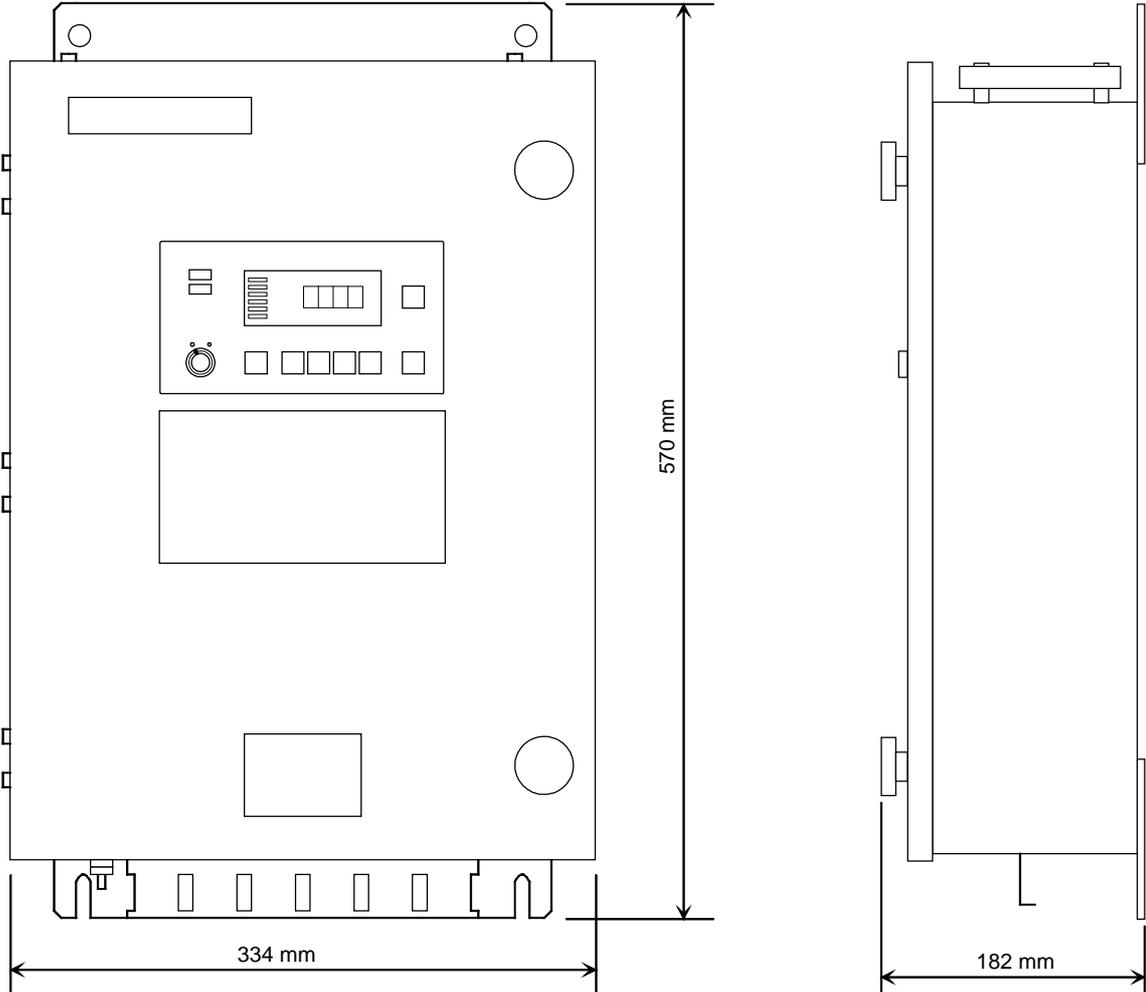
**Figure 4-3 Control Box Dimensions**
