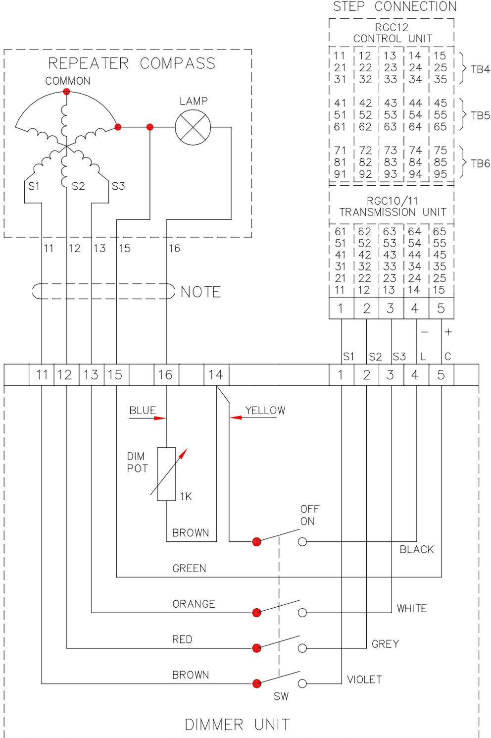
**Figure 5-8 Bearing Repeater Connection Diagram**
