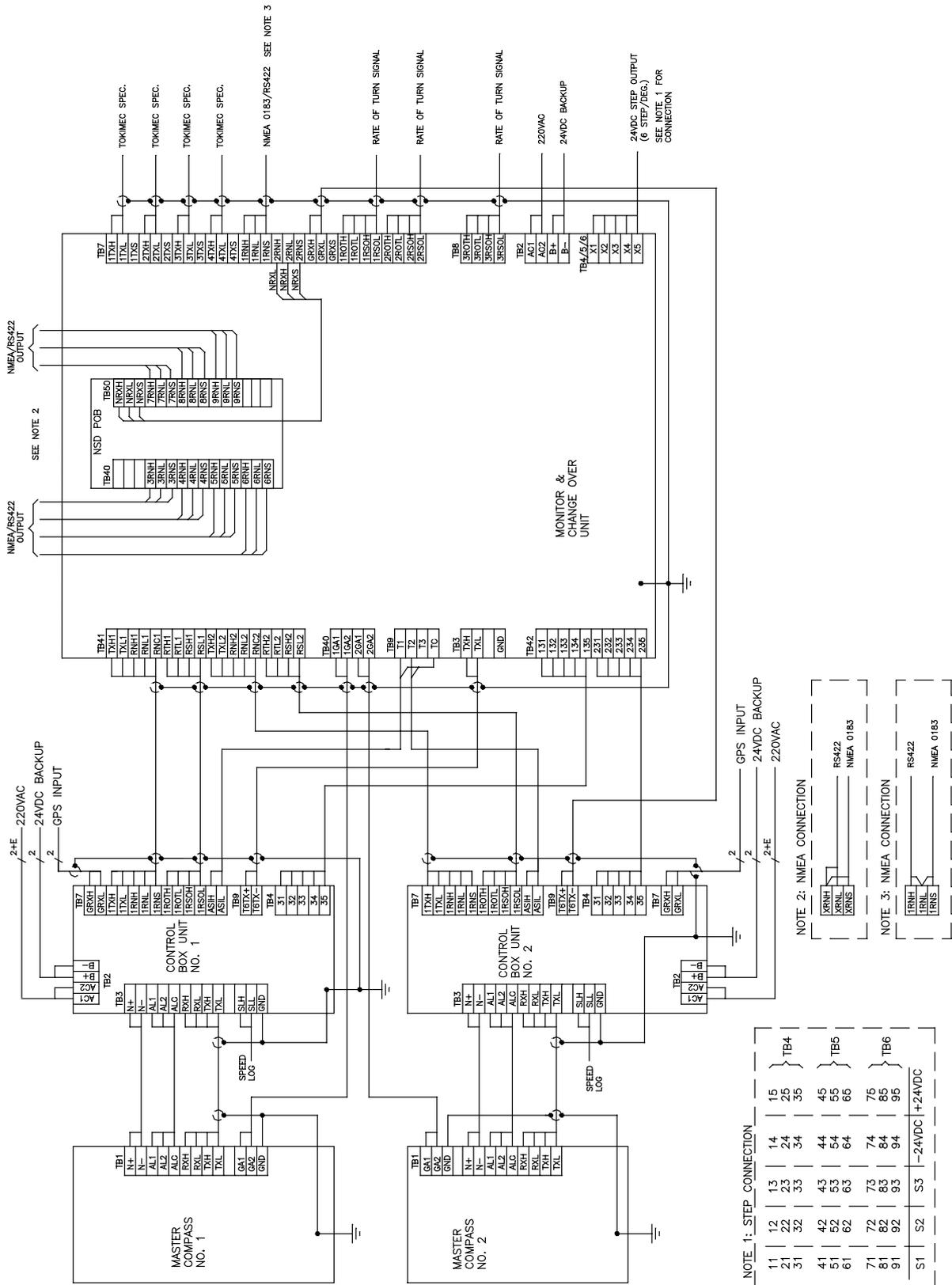
Figure 5-11 Change Over Unit - Wiring Diagram (N3-082462A)
