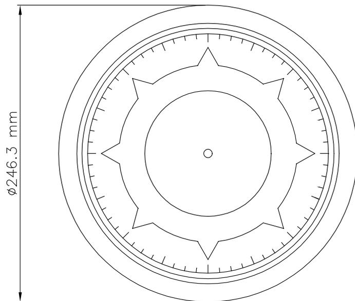
**Figure 5-5 RP-41-1 Bearing Repeater - Dimensions**
