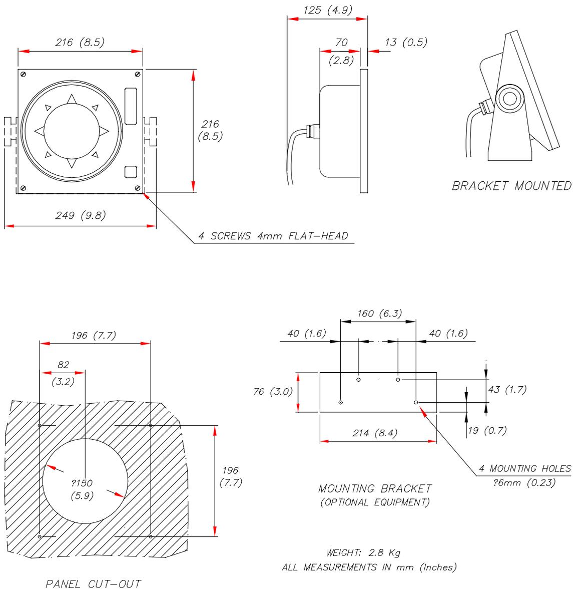
**Figure 5-3 RSR68 Steering Repeater - Dimensions**
