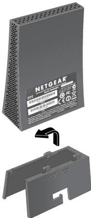
Figure 8. Attach the stand to the Internet adapter
