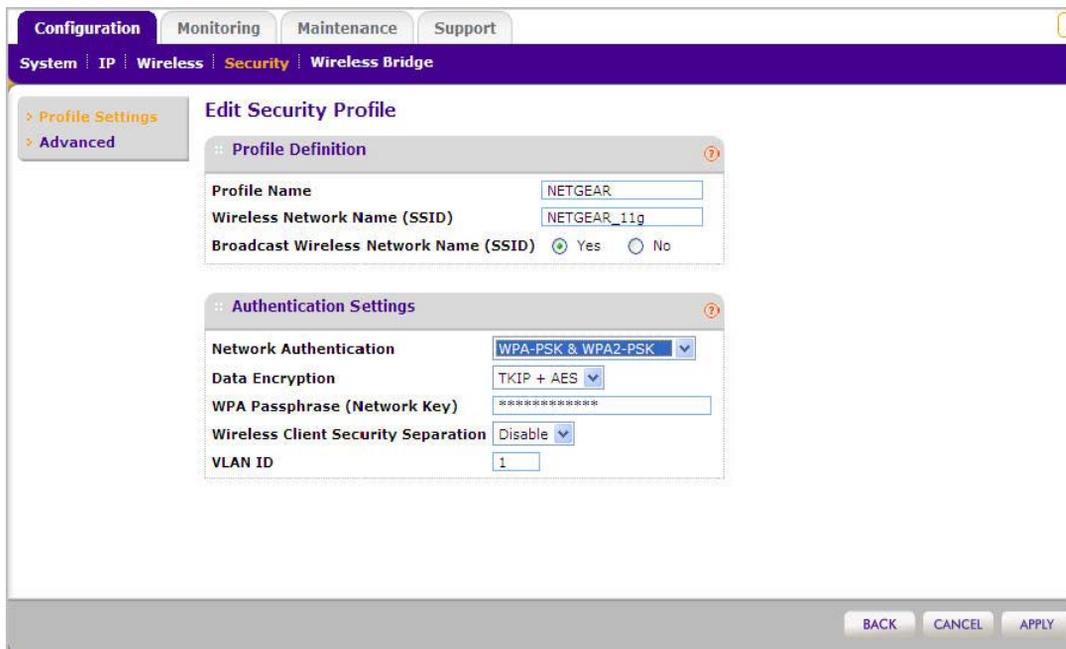
**Figure 2-23 Configure WPA-PSK and WPA2-PSK**
