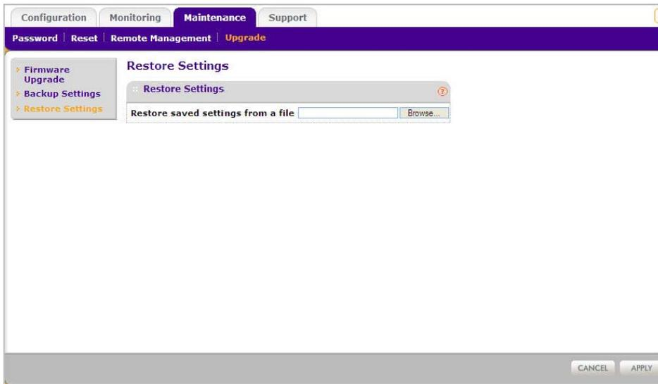
**Figure 3-6 Restore Configuration settings from file**
