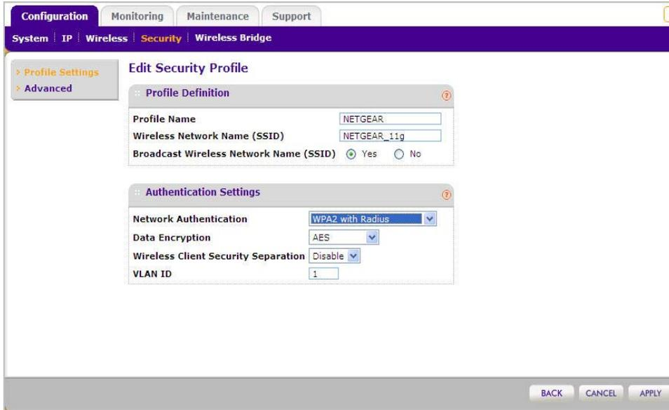
**Figure 2-19** Configure WPA2 with RADIUS
