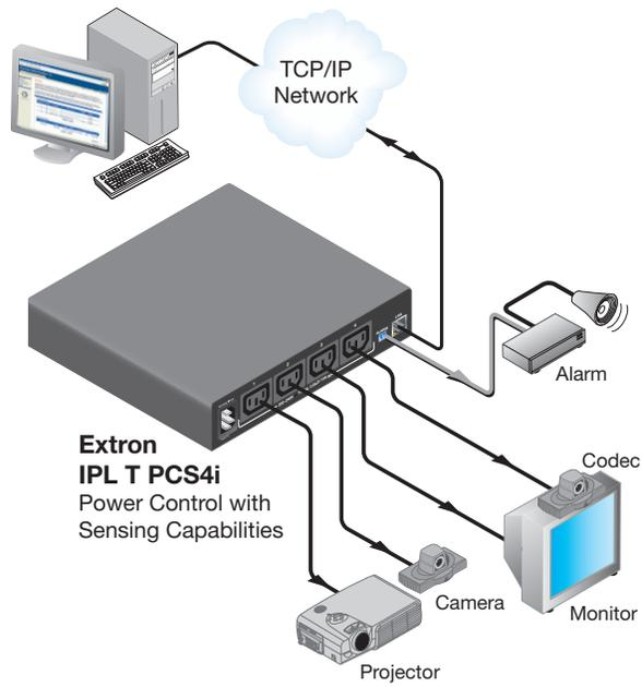
**Figure 2.** Connection Diagram for IPL T PCS4i
