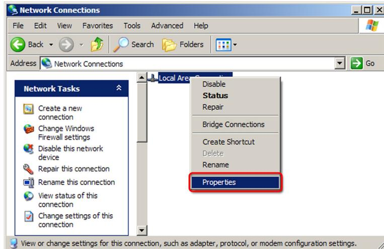
3. Select **Internet Protocol (TCP/IP)**, and click the **Properties** button. If **Internet Protocol (TCP/IP)** is not on the list, it must be added (installed). See your Windows user manual or the Windows online help system for information on how to install the TCP/IP protocol.
