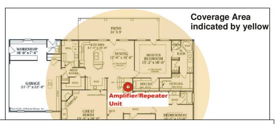
Inside Coverage area is based upon outside signal strength. A weak outside signal (-90dB) will provide less inside coverage area than a stronger outside signal (-70dB).
