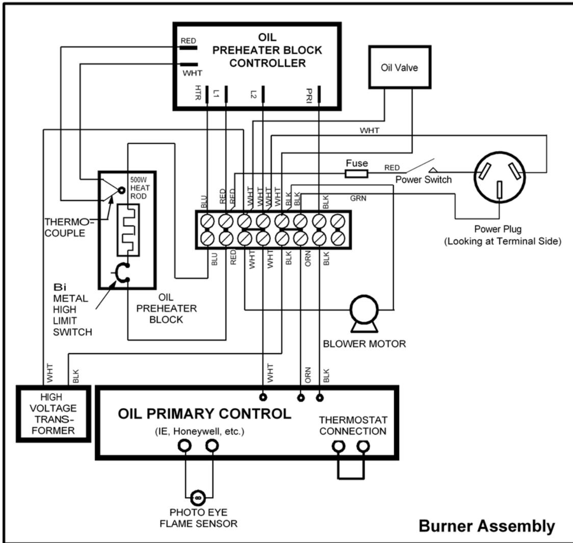
Figure 33. WIRING DIAGRAM, SINGLE HEATING ZONE ONLY
