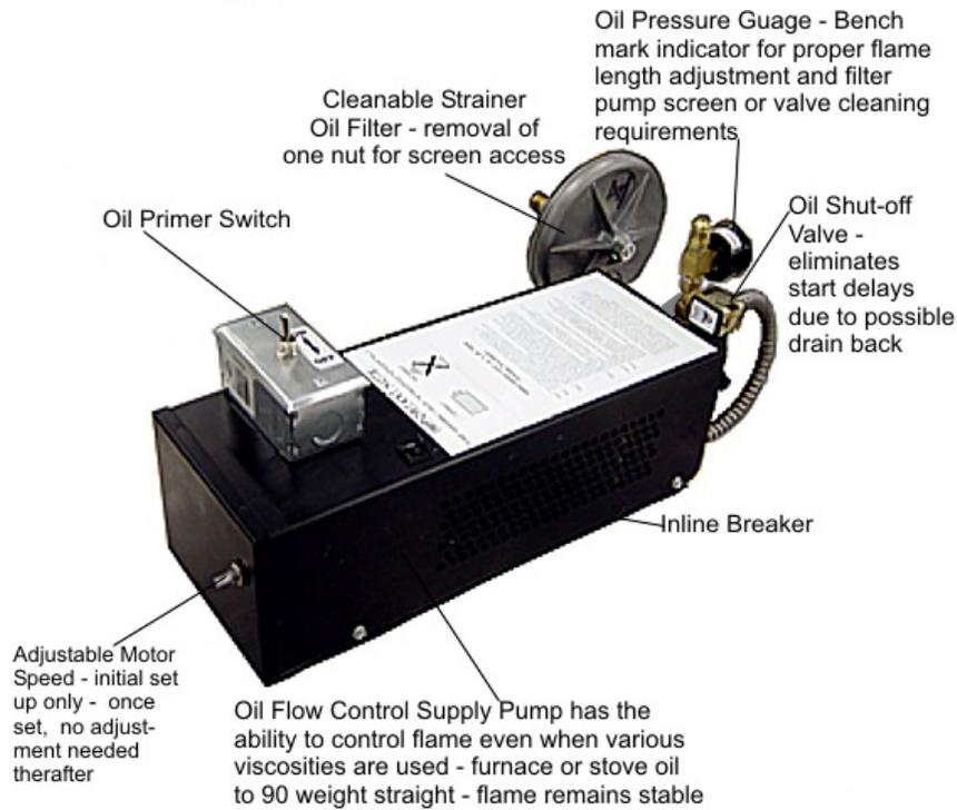
**Figure 5** –Oil Pump Assembly
