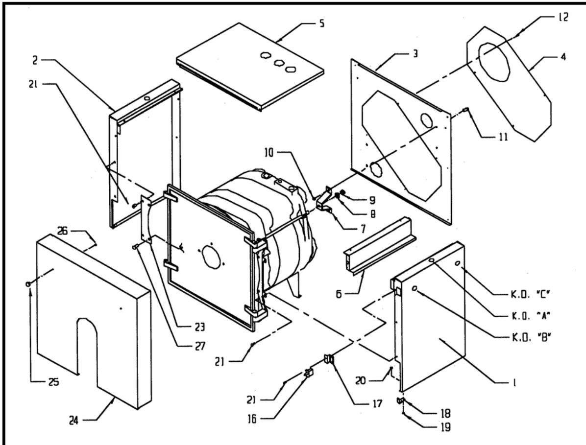
**Figure 32. OWB-9, OWB-15 and OWB-25 Assembly Detail**
