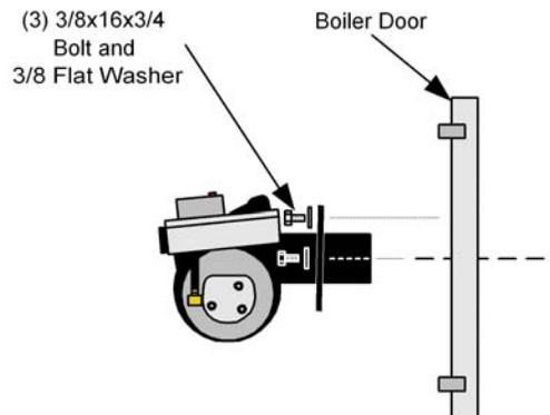
Figure 30. OWB-9, OWB-15 and OWB-25 Burner Mounting & Boiler Door Detail
