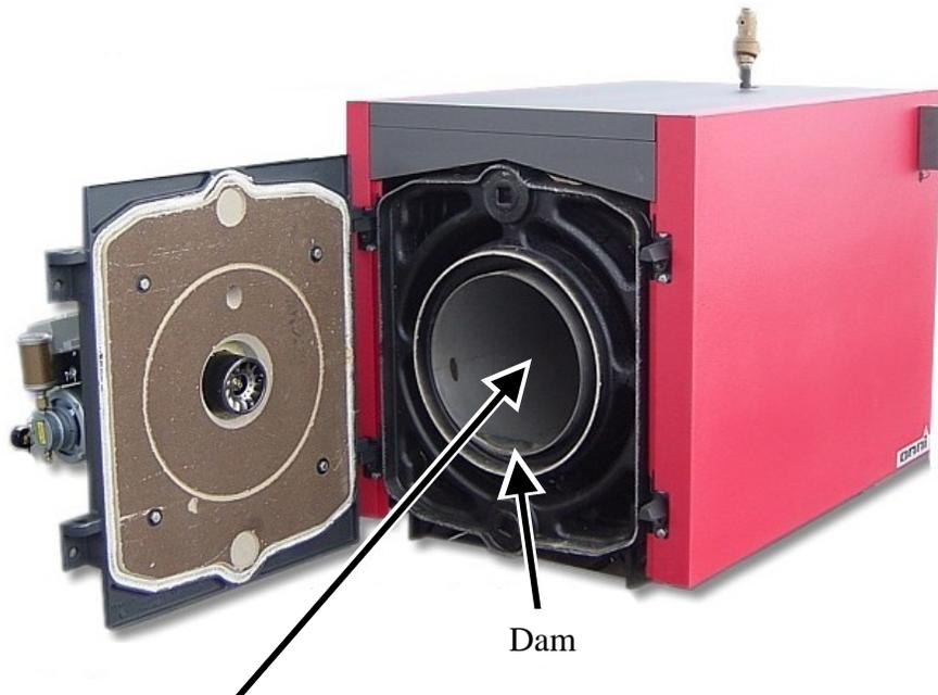
Install Stainless Steel Tube Insert with external stitch weld touching 1<sup>st</sup> water section high point of casting and the dam located at the 6 O'clock position. (bottom of boiler). When boiler door is closed, stainless tube will inbed into door refractory at least 1/4".
