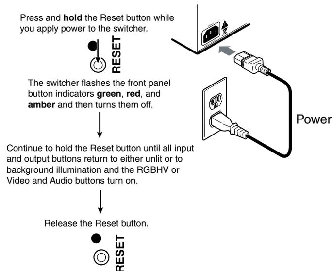
**NOTE** *The Reset button on switchers with matrix sizes of 24 x 12 and above have a different appearance and do not have a rear panel Reset LED.*
