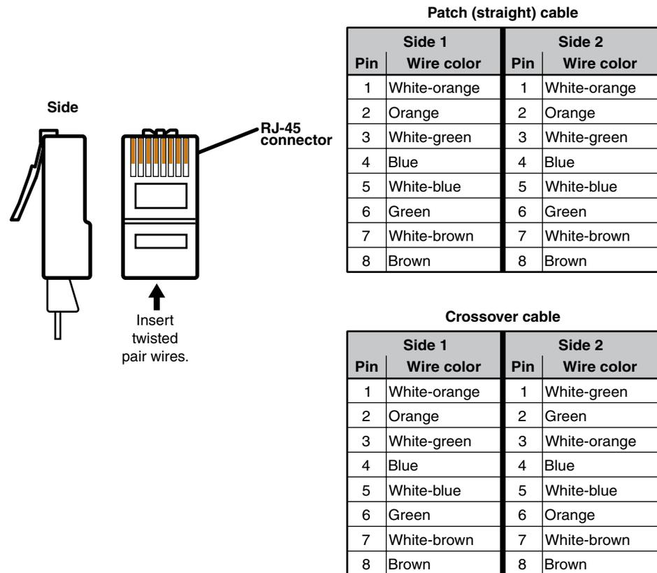
**Figure 4-3 — RJ-45 Ethernet connector pin assignments**
