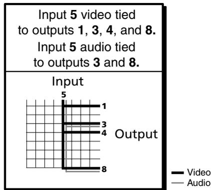
**Figure 3-22 — Example 3, final configuration, audio switcher**
