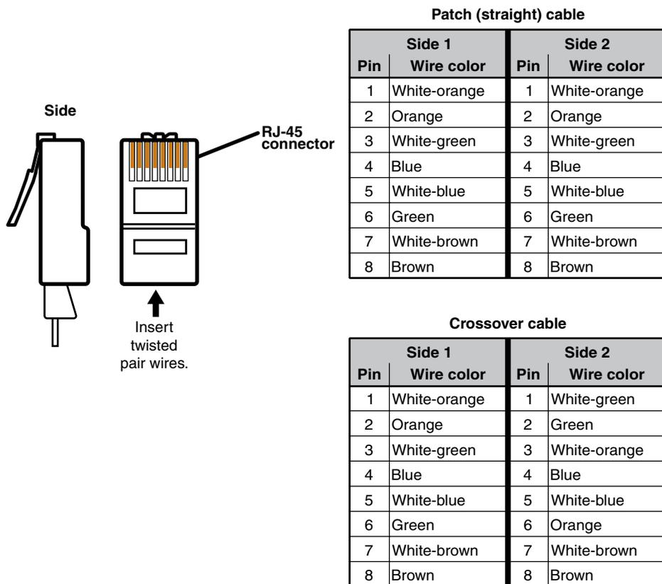
Figure 2-21 — RJ-45 connector and pinout tables
