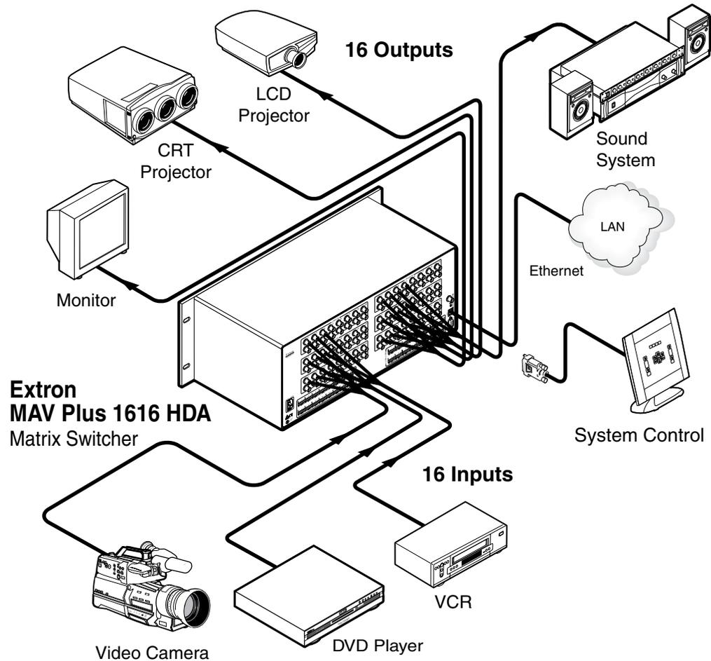
**Figure 1-2 — Typical MAV Plus matrix switcher application**
