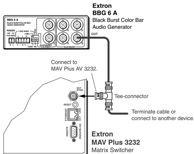
**Figure 2-22 — Simple external sync connection example**
