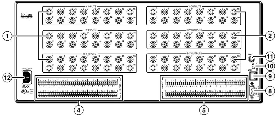
**Figure 2-7 — MAV Plus 1616 HDA matrix switcher**
