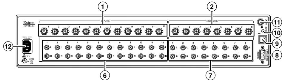
**Figure 2-9 — MAV Plus 128 AV RCA matrix switcher**
