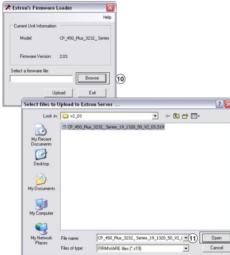
**Figure 5-12 — Firmware loading**
