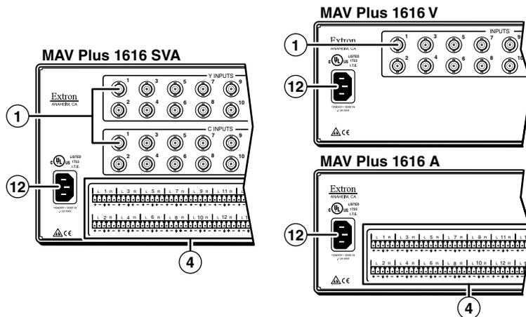
**Figure 2-8 — MAV Plus 1616 matrix switchers with various formats**
