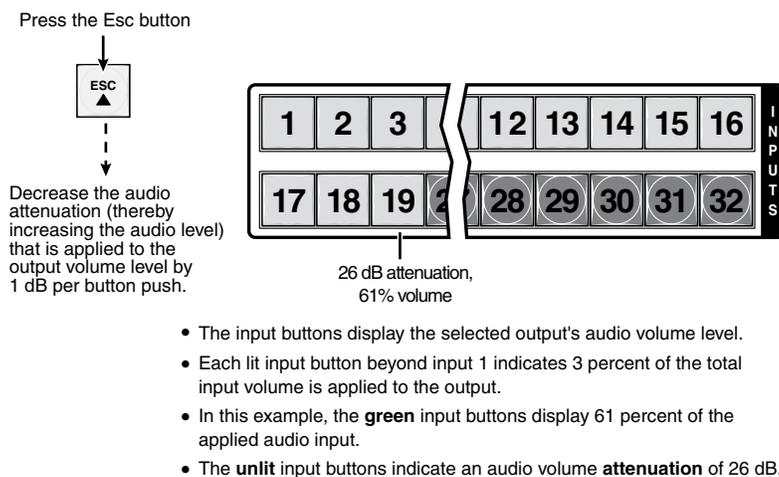
**Figure 3-71 — Adjust the output audio volume**
