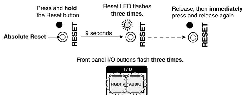
**NOTE** The Reset button on switchers with matrix sizes of 24 x 12 and above have a different appearance and do not have a rear panel Reset LED.
