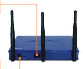
2. Connect the AC Power Adapter to the Access Point and then to a power outlet.
