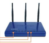
Verify that the following front panel lights are on: Power, LAN and WLAN.
