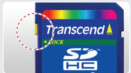
Mechanical write-protection switch
