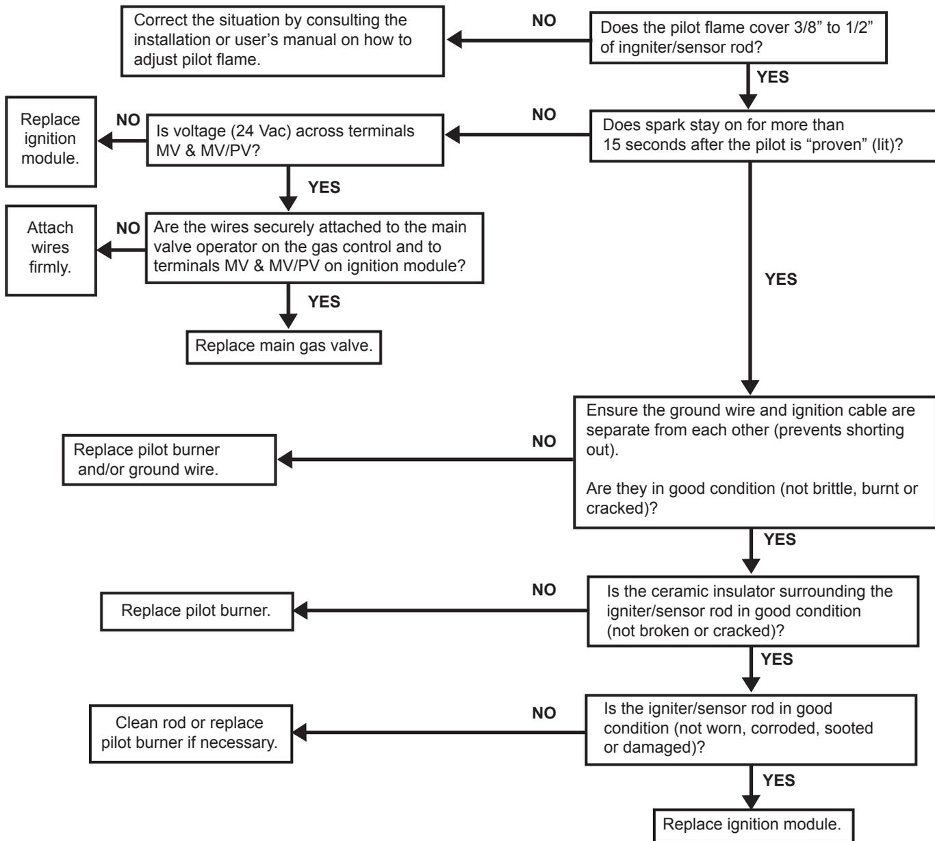
**CHECKING HONEYWELL S8600H OR S-8610M
