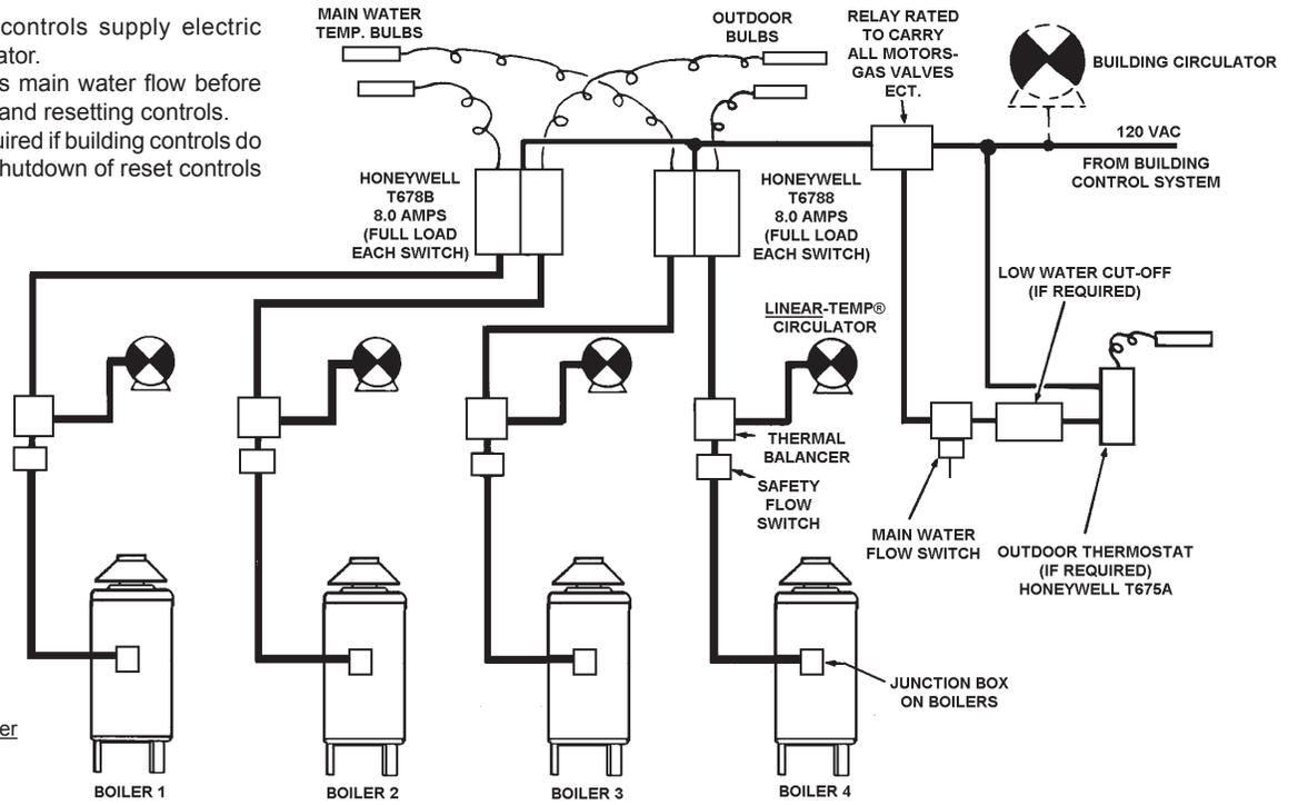
Boilers and Secondary Circulator are Controlled by Dual Bulb, Dual Switch Controller Staging and Outdoor Reset of Main Water Temperature
