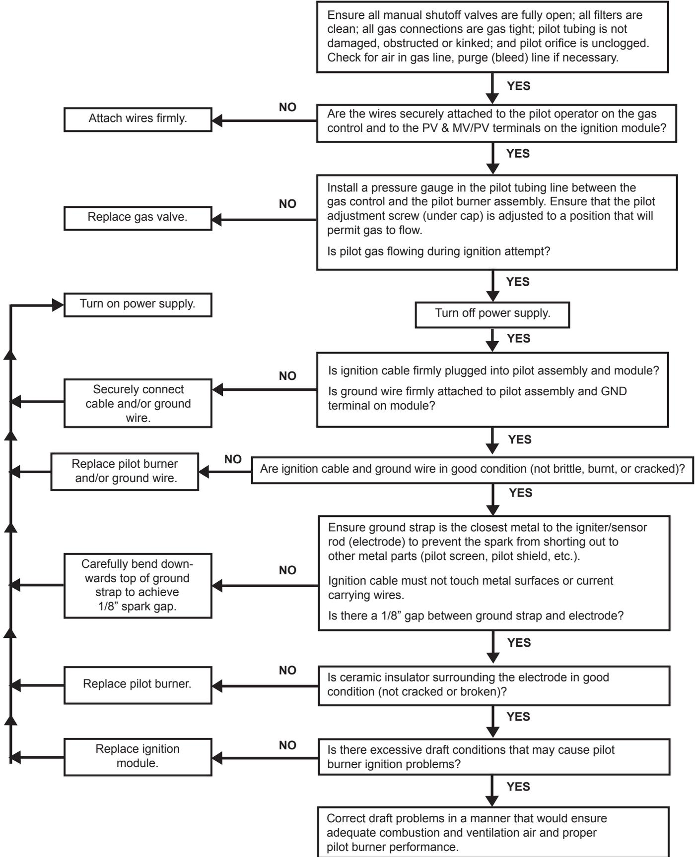
**CHECKING HONEYWELL S-8600H OR S8610M
