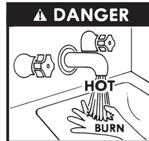
The tank temperature control is adjustable from 100°F (37.7°C) to 220°F (104.4°C). It is recommended that lower water temperatures be used to avoid the risk of scalding. It is further recommended, in all cases, that the water temperature be set for the lowest temperature which satisfies the user's hot water needs. This will also provide the most energy efficient operation of the water heater and minimize scale formation.
