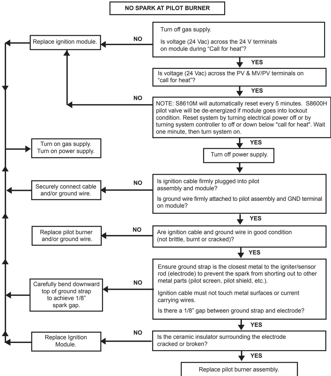
**CHECKING HONEYWELL S8600H OR S-8610M
