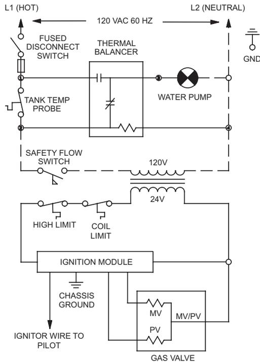
**NOTE:** IF REPLACING ANY FACTORY WIRING, USE TYPE 105°C WIRE OR EQUIVALENT, EXCEPT FOR THE IGNITION WIRE WHICH USES 250°C WIRE AND THE COIL LIMIT WHICH USES 200°C WIRE.
