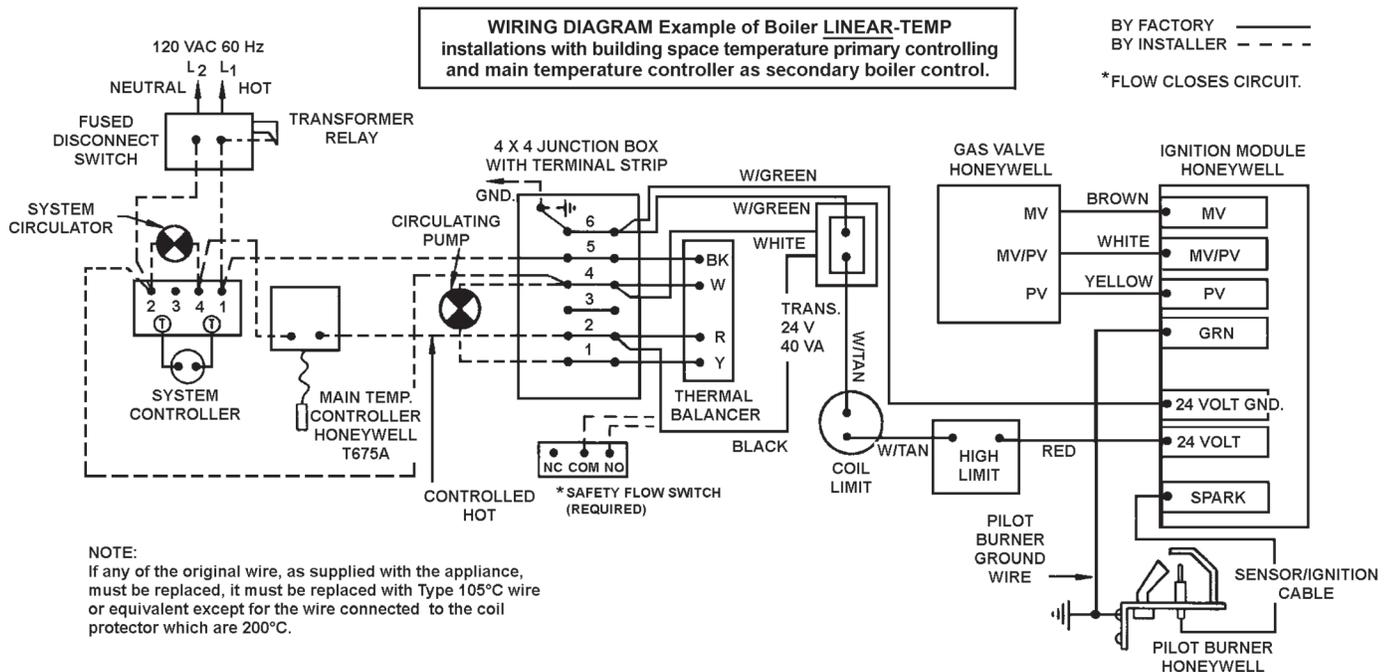
**TYPICAL WIRING DIAGRAM (IID SYSTEM) FOR SINGLE BOILER LINEAR-TEMP® INSTALLATION
