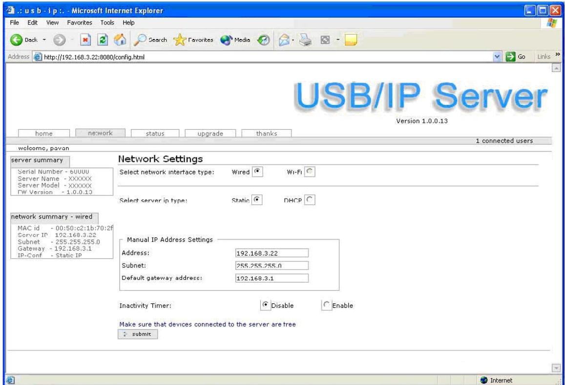
For the wired interface you can configure the Static IP, Subnet Mask, and Gateway manually or set the box to automatically obtain an IP address by setting to the Dynamic (DHCP) mode.
