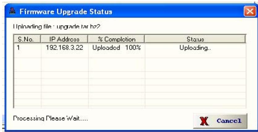
As soon as the transfer is completed, the USB device server automatically restarts to apply the upgraded firmware settings.
