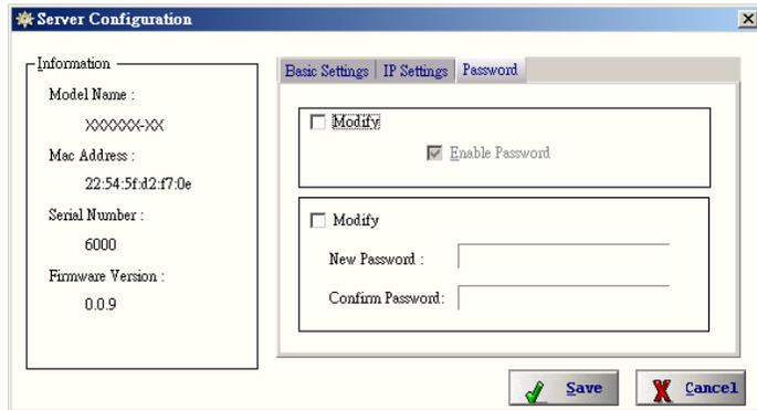
Check the Modify box to Enable or Disable password option to the USB device server.
