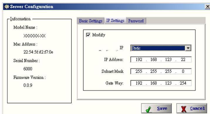
After entering IP address, Subnet Mask & Gate Way then click on “save” button. Then USBIP Admin shows progress bar for some time and after it pops up a message box as shown below.
