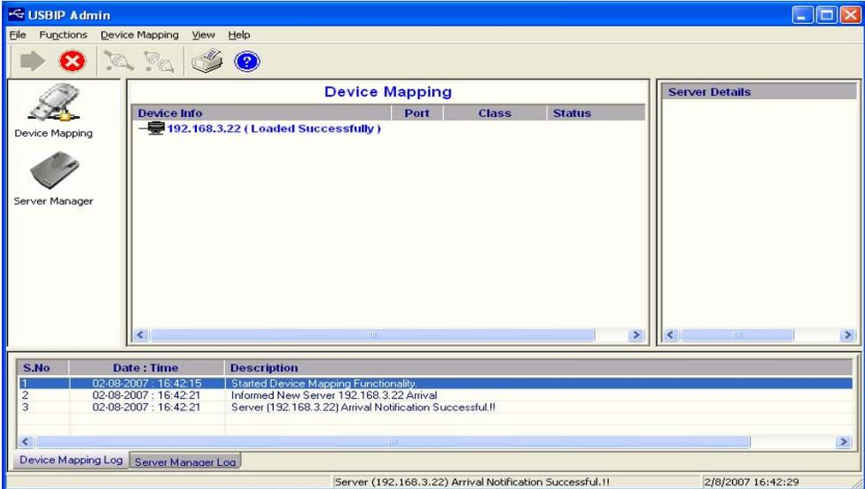
In the Device mapping window, all the USB devices connected are shown as a tree under the USB Server. Right click on any device and click on “Connect” to virtualize that USB device onto your PC as shown below.
