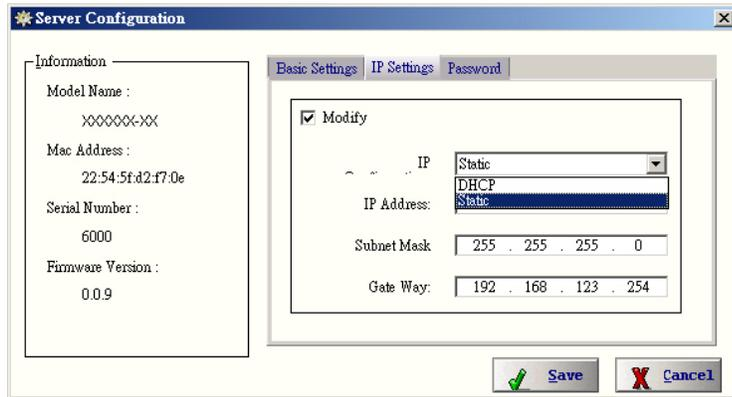
After Selecting IP Configuration key in the IP Address of the USB device server in the IP Address field followed by proper Subnet Mask & Gate Way as shown below.
