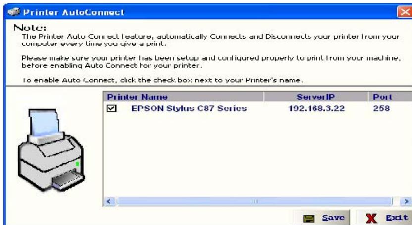
Select the Printer which was connected and Click on “Save” and close the Window.
