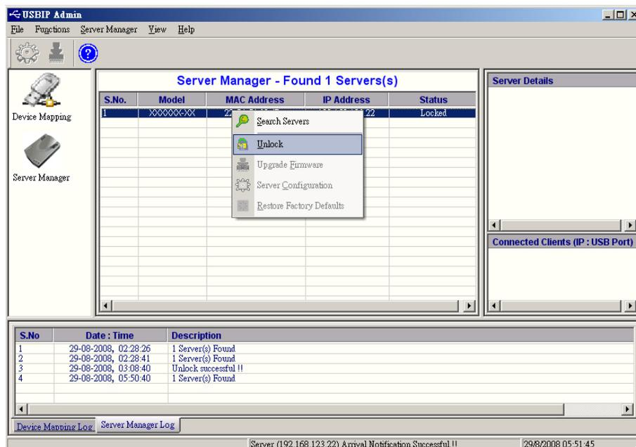
On selecting 'Un-Lock' the password dialog pops up as shown below. Key in the password in the 'Password' dialog. The default password for the USB IP Server is "usbip"
