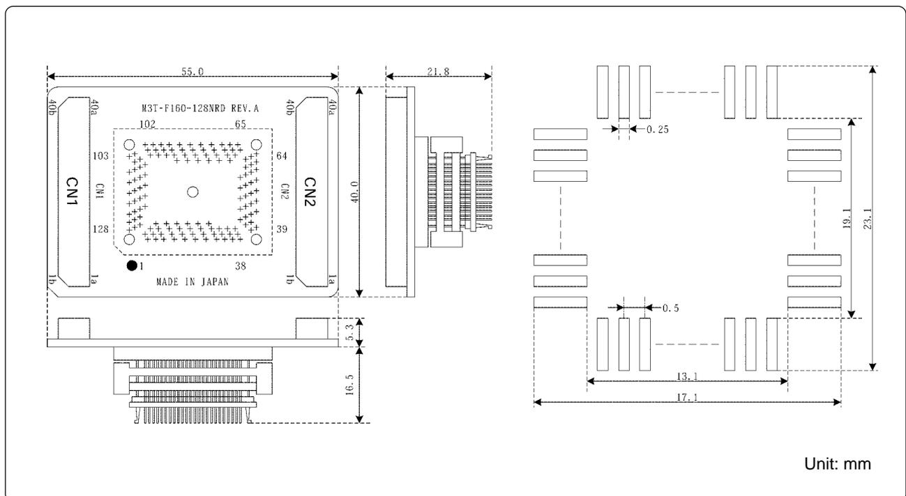
Figure 4 External dimensions and a sample foot pattern
