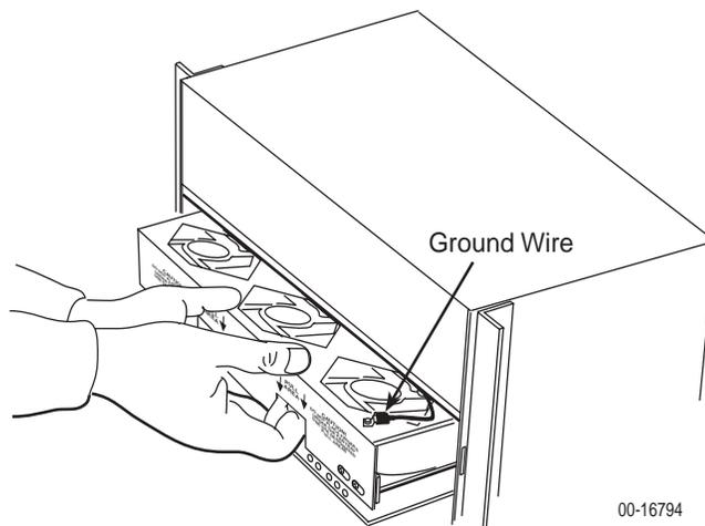
4. **Wait until the fan blades stop spinning** (which should be less than a minute). Disconnect the ground wire attached to the fan tray bracket, from the quick connect terminal on the chassis.
