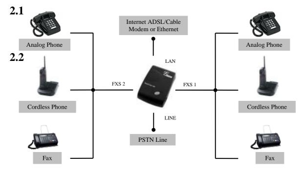
HandyTone-386 has two FXS ports. The RJ-11 jack next to the LAN is called FXS port 2 and the RJ-
