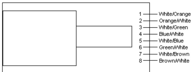
**Figure C-3: Gigabit straight-through wiring for RJ-45 connector**
