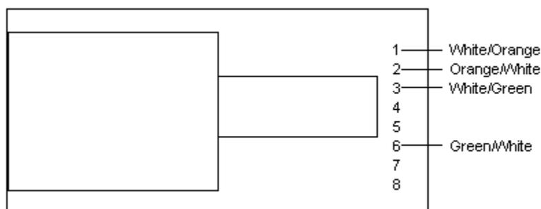
**Figure C-1: 10/100 straight-through wiring for RJ-45 connector**
