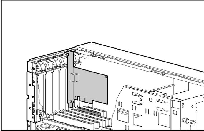
**Figure 2-1: Installing the adapter in a server**
