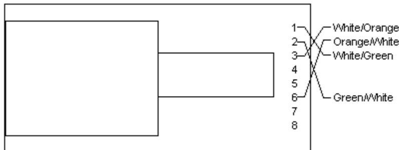
**Figure C-2: 10/100 external crossover for RJ-45 connector**
