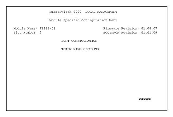
Figure 4. 9T122-08 Module Specific Configuration Menu Screen
