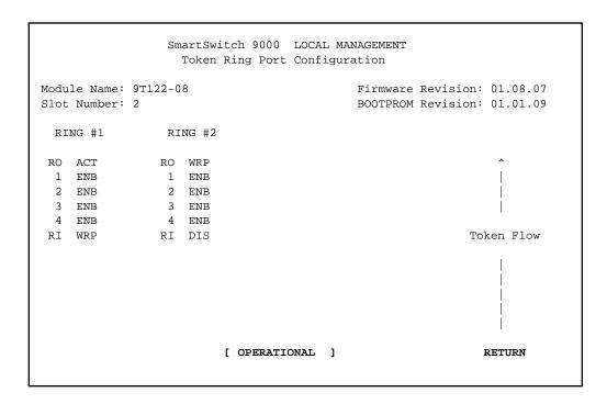
Figure 5. 9T122-08 Token Ring Port Configuration Screen
