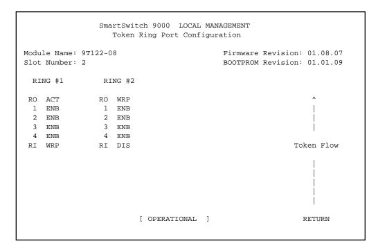
Figure 7. 9T122-08 Token Ring Port Configuration Screen (Operational Mode)
