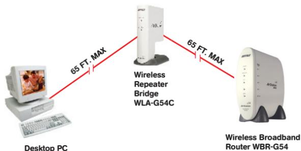
**Figure 3:** Basic placement of repeater with repeater approximately half way between client machine and the router (65 feet from router to repeater and 65 feet from repeater to computer).
