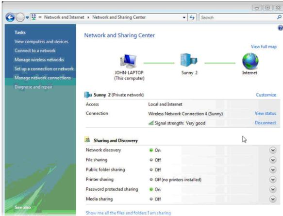
**A.15** The Network and Sharing Center now indicates the network connection that you have just made. The links on the left of the window allow you to configure your network connections.
