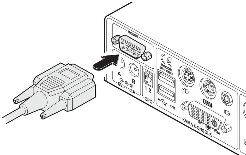
*Note: The default serial port speed is 115200 and a standard Hayes-compatible auto-answer string is sent during startup. The default startup string is 'ATZHS0=1'. Both the serial port speed and startup string settings can easily be altered during the local or remote configuration - see [Initial configuration](#) for more details. The other serial settings are fixed at: No parity, 8 bit word and 1 stop bit.*
