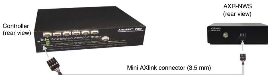
**FIG. 7** AXR-NWS connection to a Controller
