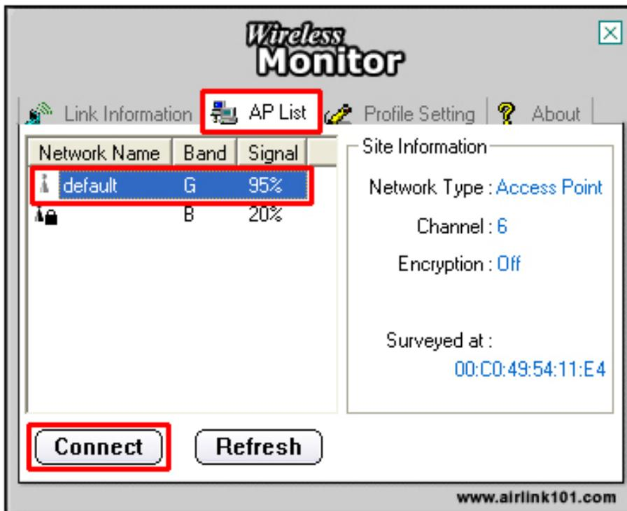
**Step 2** If encryption is not enabled for the selected access point / router, skip to Step 6. Otherwise, enter a **Profile Name** for your wireless setting and click **Next**.
