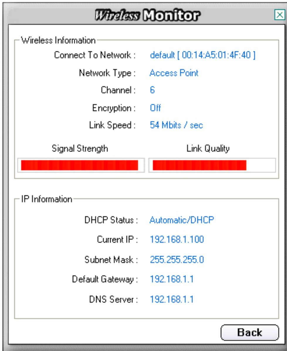
The Wireless Information displays the current wireless network you are connected to as well as various other statuses such as the Signal Strength and your assigned IP address.
