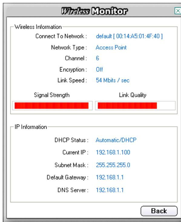
If you do not have adequate Signal Strength, try re-orienting the Access Point and/or the USB Adapter to get a better reception.
