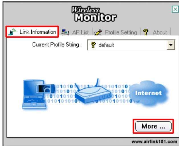
**Step 8** Verify that you are receiving adequate Signal Strength and Link Quality and that you have been assigned a valid IP address (instead of all 0's).
