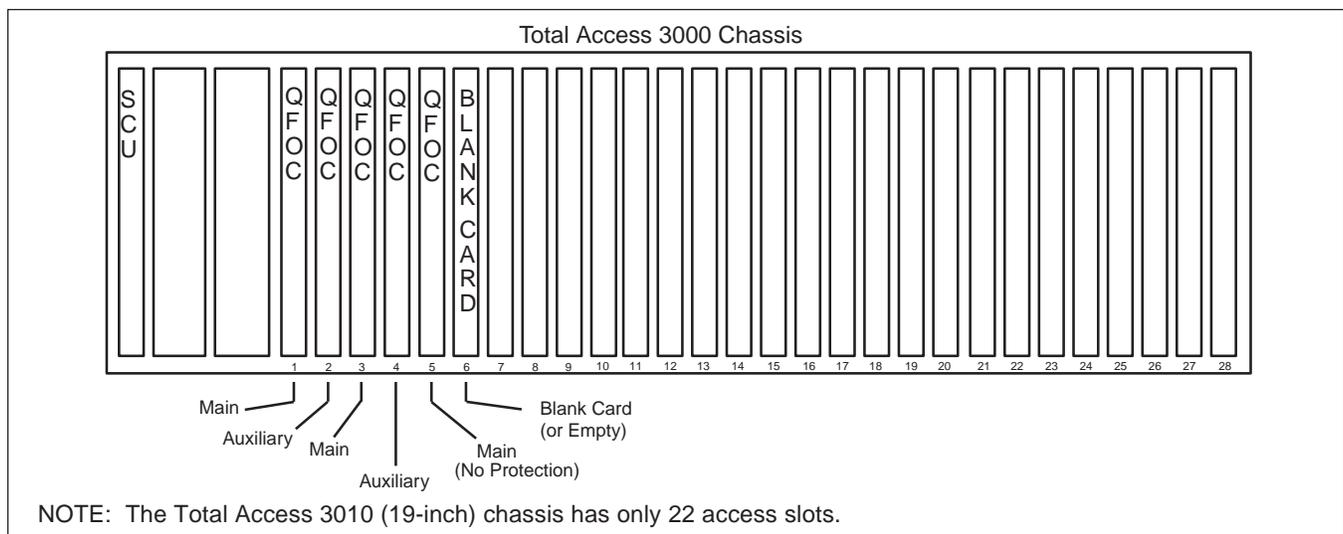
Figure 2. Total Access 3000 CO Chassis
