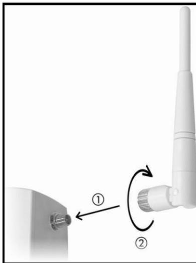
**Figure 23 Attaching Antennas**
