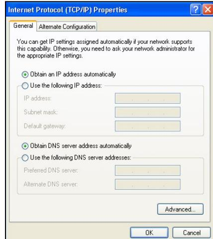
6. Click **Advanced**. Remove any previously installed gateways in the **IP Settings** tab and click **OK** to go back to the **Internet Protocol TCP/IP Properties** screen.
