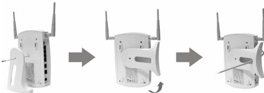
**Figure 24 Support Holder Connections**
