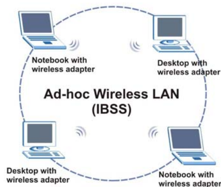
Figure 2-1 Ad-hoc Network Example
