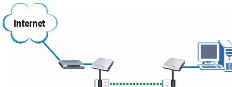
Connect your PLA-4xx to an Internet gateway such as a modem and plug it into an ordinary power outlet in your home. Plug a second PLA-4xx into another power outlet and connect a computer to the PLA-4xx for Internet access. Your network can be further expanded by plugging additional PLA-4xxs into other outlets in your home and connecting other computers or network devices (for example, a printer) to them.
