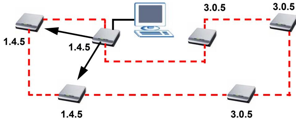
This diagram shows the **Firmware Detection Tool** detecting the firmware on latest firmware devices only, as the local device has the latest firmware.
