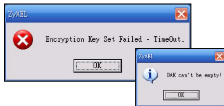
Figure 29 Incorrect DAK or No DAK
