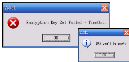
Figure 41 Incorrect DAK or No DAK
