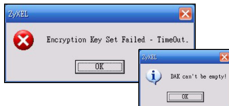
Figure 40 Incorrect DAK or No DAK
