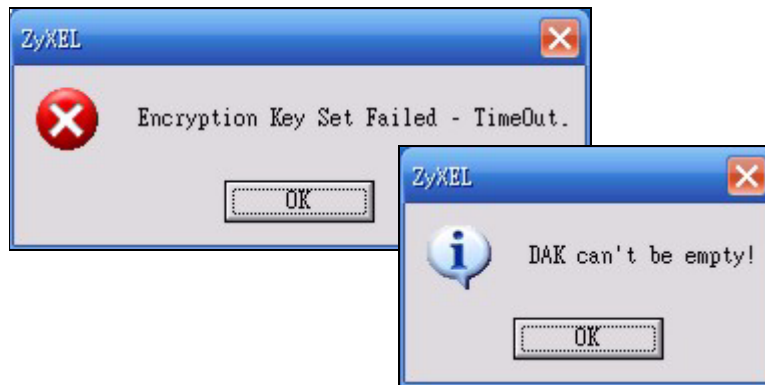
Figure 46 Incorrect DAK or No DAK
