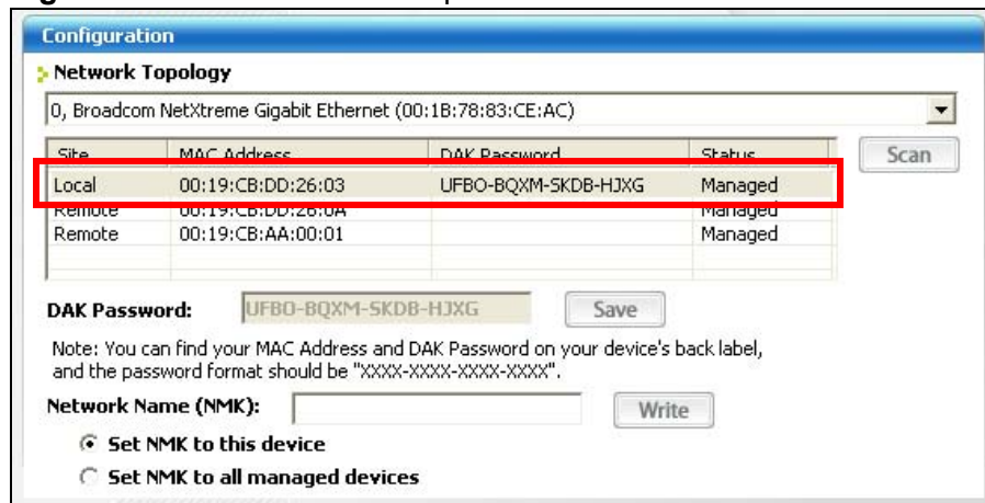
Figure 44 Local/Remote Adapters on a Powerline Network
