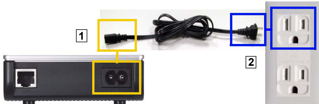
Figure 18 Plug Your Powerline Adapter into a Power Socket
