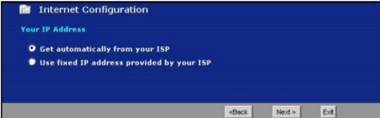
The screenshot shows a window titled "Internet Configuration" with a sub-header "Your IP Address". There are two radio button options: "Get automatically from your ISP" (which is selected) and "Use fixed IP address provided by your ISP". At the bottom are three buttons: "<Back", "Next >", and "Exit".
