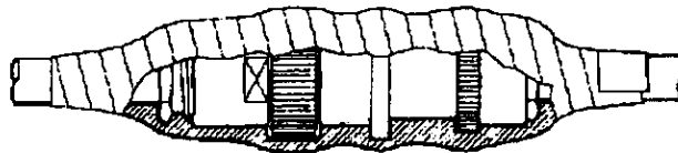
Waterproofing the antenna connector
