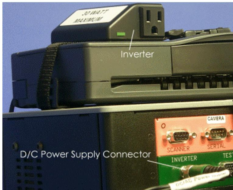
Figure 5 Power Inverter Panel
