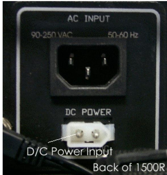
Figure 4 External D/C Power Input
