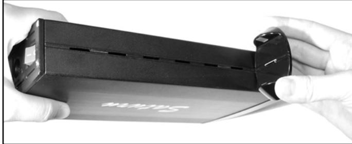
Place the Rubber Stands on the downside of the VPA-3528Net NetWork Storage, and position the Rubber Stand Location Positioner into the Rubber Stand Location Holes on the downside of the NetWork Storage.
