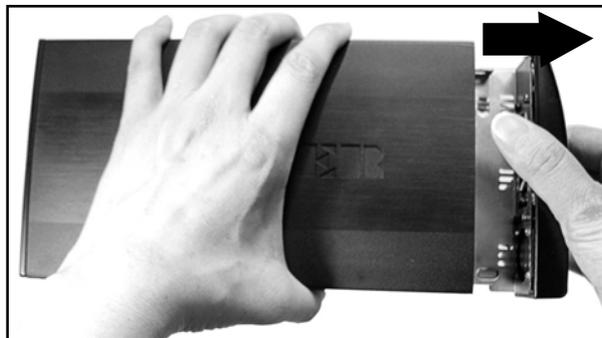
Carefully slide the **Inner Cradle with PCB and Front Cover** off the **Body Outer Cover with Rear Panel**.
