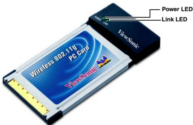
**Power LED** - This indicator will light up when the PC Card Adapter is powered on.
