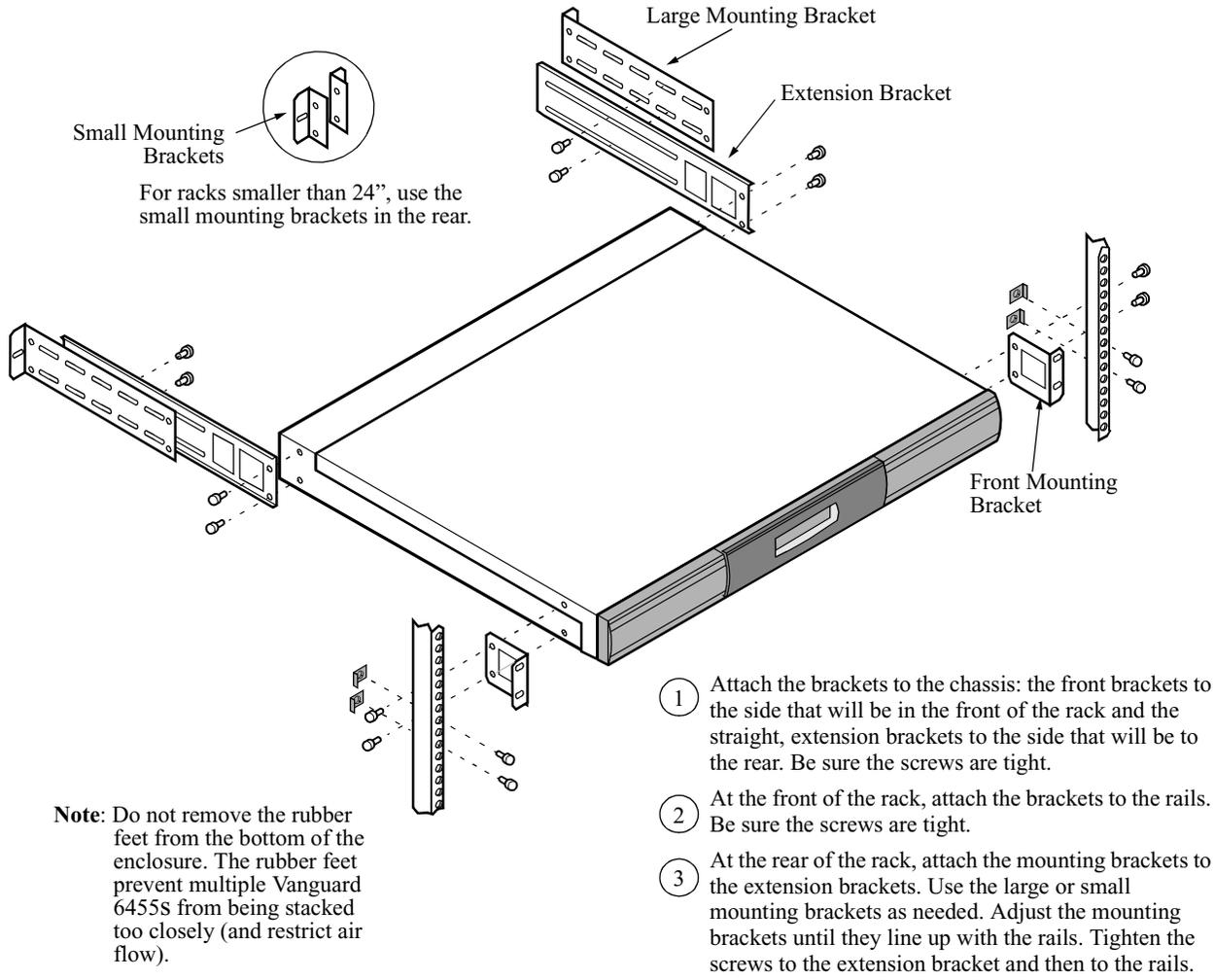
Figure 3-3. Installing the Vanguard 6455 Into a Rack
