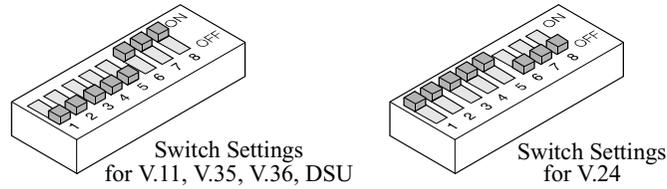
**Figure 2-7. Settings for DIM DIP Switches**
