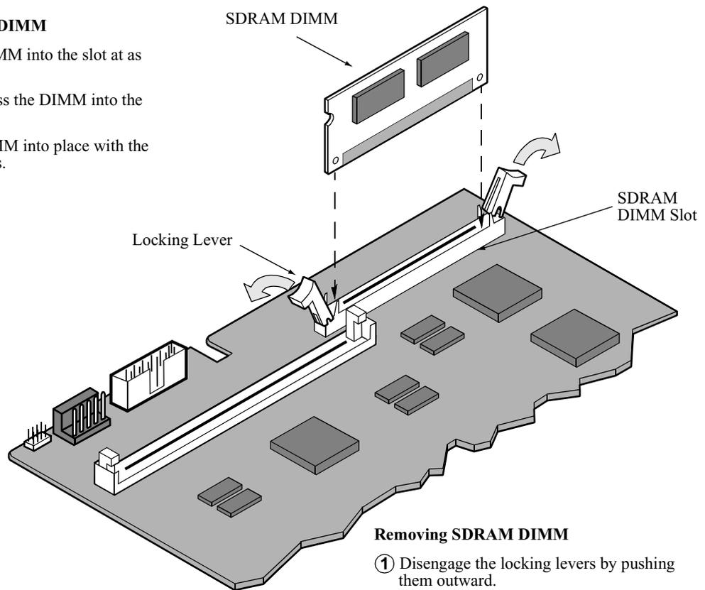
**Removing SDRAM DIMM**
