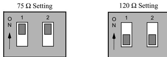
**Figure 2-42. E1 Impedance DIP Switches**
