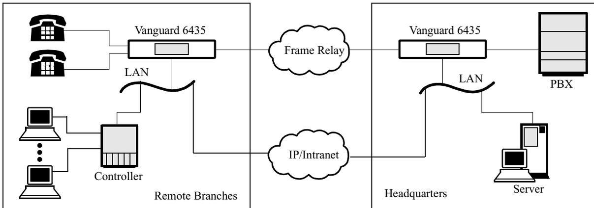
**Figure 1-4. Voice over Frame Relay or Voice over IP**
