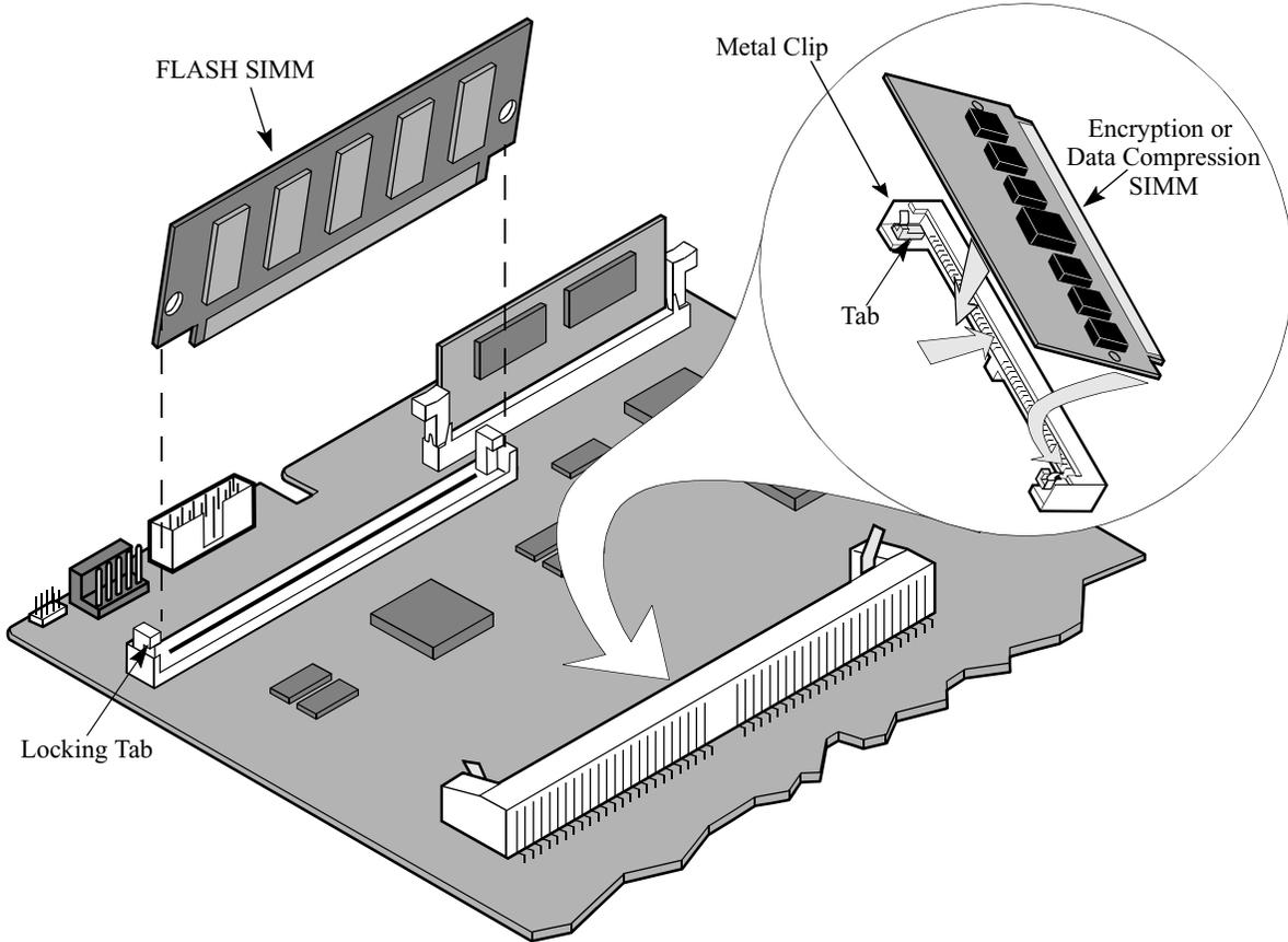
**Figure 3-13. FLASH|Data Compression|Encryption SIMM Installation**
