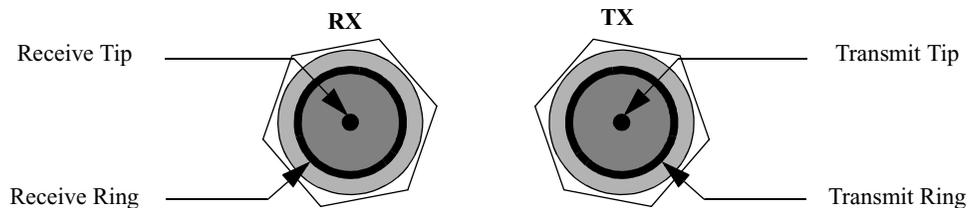
**Figure 2-41. BNC Connector: RX and TX**
