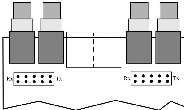
**Figure 2-43. E1 Card Impedance Jumper Locations**
