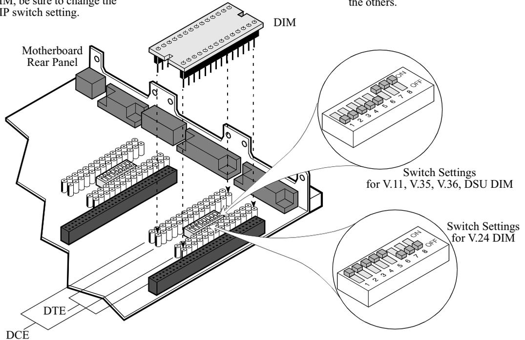
**Figure 3-11. DIM Replacement and Switch Settings**
