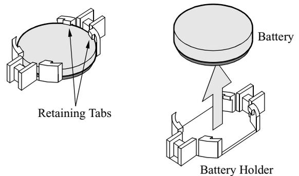
**Figure 3-16. Replacing the Battery**
