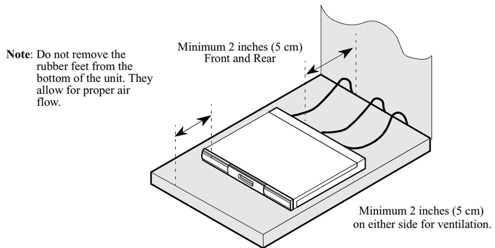
**Figure 3-2. Proper Cable and Air Clearance**
