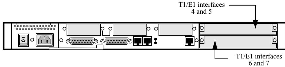
**Figure 2-37. VoIP Convergence Card Interface Assignments**
