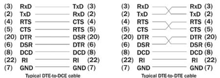
Figure 13 - illustrates the RS232 pinouts for typical DTE- to-DCE and DTE-to-DTE cables with 9-pin connectors.
