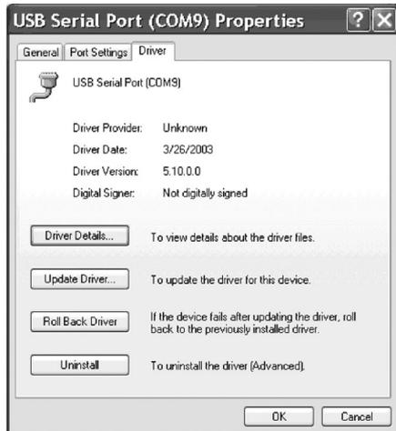
Figure 18 - Windows XP/2000 USB serial port properties, Driver box.
