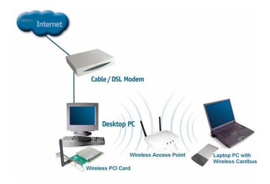
Please note that this type of installation requires that your ISP (Internet Service Provider) provide you a static IP address for each computer and the Access Point on your network. Please refer to the manual that came with your Access Point to determine its configuration.
