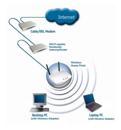
(Requirements: A Residential Gateway/Router connected with an Ethernet (CAT5) cable to an 802.11a/b Access Point or an 802.11a/g Access Point or another computer with an 802.11b/g WLAN card installed).
