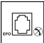
**EPO (Emergency Power Off) Port:** Your UPS features a EPO port that may be used to connect the UPS to a contact closure switch to enable emergency inverter shutdown. See Optional Installation.
