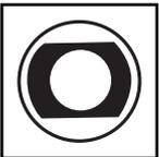
**Output Breaker (select models):** Your UPS features one or more breakers that protect your UPS from output overload. If one or more breakers trip, remove some of the load on the circuit(s), then reset them by pressing the breaker switch(es) in.
