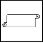
**Accessory Slot:** Remove the small cover panel from this slot to install optional accessories to remotely monitor and control your UPS. Refer to your accessory's manual for installation instructions. Contact Tripp Lite Customer Support at (773) 869-1234 for more information, including a list of available SNMP, network management and connectivity products.
