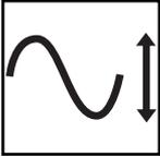
**“VOLTAGE CORRECTION” LED:** this green LED lights continuously whenever the UPS is automatically correcting high or low AC voltage on the utility line without the assistance of battery power. The UPS will also emit a slight clicking noise. These are normal, automatic operations of the UPS, no action is required on your part.
