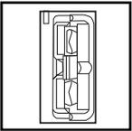
**External Battery Connector (Select Models Only):** Use to connect Tripp Lite external battery packs for additional runtime. Refer to instructions available with the battery pack for complete connection information and safety warnings.
