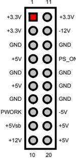
If the system is not using the ATX power function, you may SHORT pins 4 and 5 of CN10 so that the ATX power supply can be used as an AT power unit. If not, CN2 must be connected to a corresponding connector on a PICMG Bus backplane in order to use the ATX Power function.
