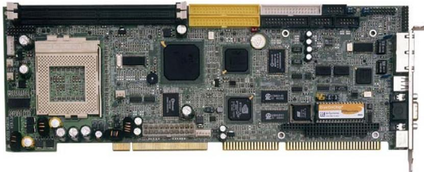
The HS-6038 is a 133MHz FSB Intel® 82815/82801BA chipset-based board designed for PICMG Bus Celeron™/Coppermine™/Tualatin™ 800MHz~1.2GHz CPU compatibility. These features combine and make the HS-6038 an ideal all-in-one industrial single board computer. Additional features include an enhanced I/O with CompactFlash, VGA, dual LAN, audio, and two COM interfaces.
