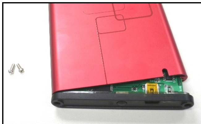
Figure 3. Remove the top cover revealing the IDE/SATA adapter
