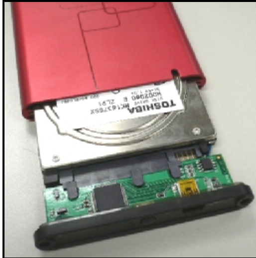
Figure 5. Reinsert the adapter plus drive and reattach the screws
