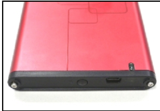
Figure 2. Remove the screws from the top cover
