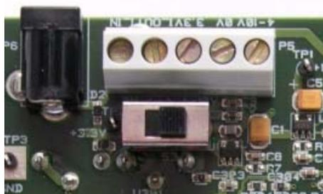
**Figure 3: SmartRF04EB Power switch, power on.**
