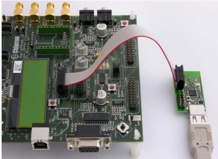
**Figure 1 CC2511 Dongle powered from USB cable**
