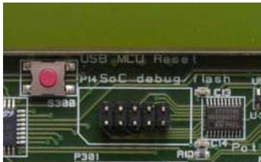
Figure 5: SmartRF04EB debug connector for debugging
