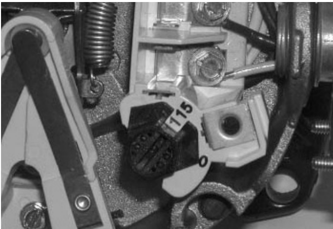
Figure 13: Motor Set for 115 Volt Operation
