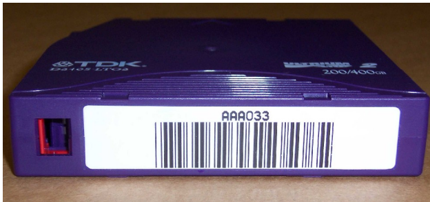
Figure 13. Positioning of Barcode Label for LTO Cartridges
