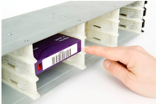
Figure 20. Push the Release Knob towards the Cartridge to Eject the Cartridge from the Slot
