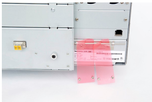
Figure 4. Recommended Storage of Transport Locking Screws
