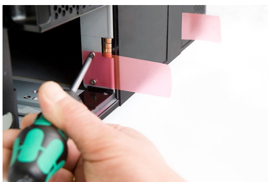
Figure 3. Transport Locking Screws Marked with Red Plastic Tabs
