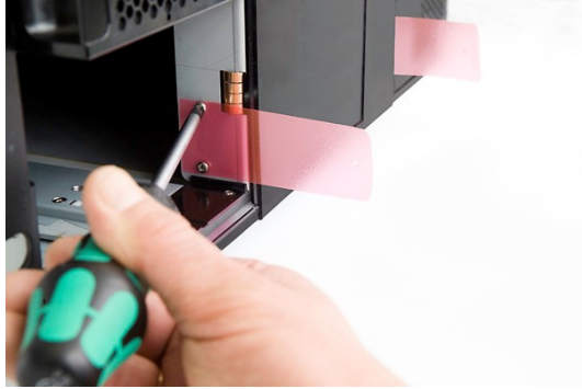
Figure 25. Transport Locking Screws Marked with Red Plastic Tab
