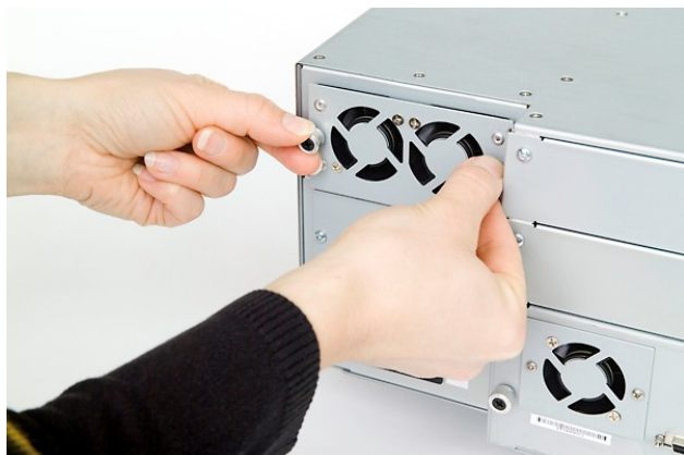
Figure 23. Replacing a Power Supply
