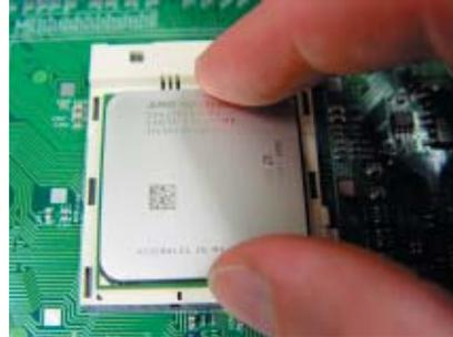
4. With the CPU inserted into the socket, inspect the four corners of the CPU to make sure that it is properly installed and flush with the socket.
