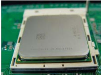
5. Gently press the CPU socket lever down until it locks in the plastic tab.
