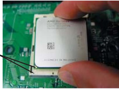
3. Align pin 1 of the CPU with pin 1 of the socket. Once aligned, carefully place the CPU into the socket. *Do not drop the CPU on the socket, move the CPU horizontally or vertically or rub the CPU against the socket or against any pins of the socket, which may damage the CPU and/or the socket.*
