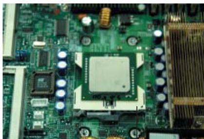
Socket lever in the locked position
