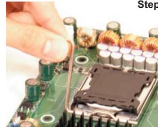
8. If the CPU is properly installed into the socket, the black plastic cover will be automatically released from the load plate when the lever is pushed into the hook. Remove the cover from the motherboard.
