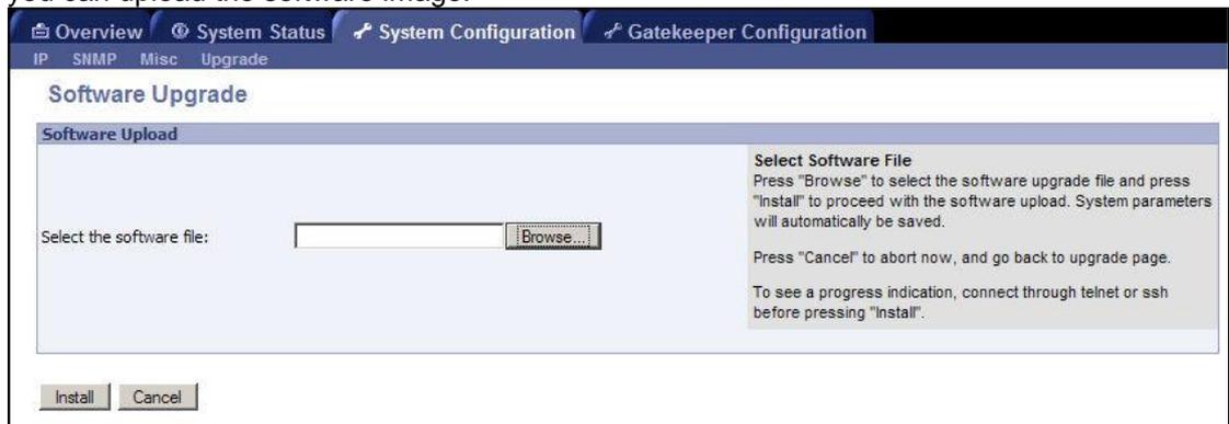
5. Browse to the file containing the software and press Install. You should see a page indicating that upload is in progress:
