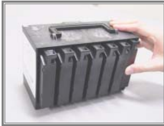
Figure 3-6 Removal and Insertion of Cartridges (7-Slots)
