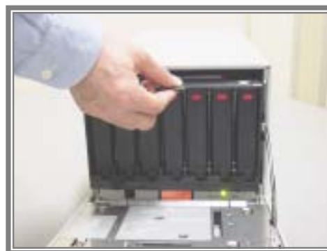
Figure 3-2 Pulling out the Magazine
