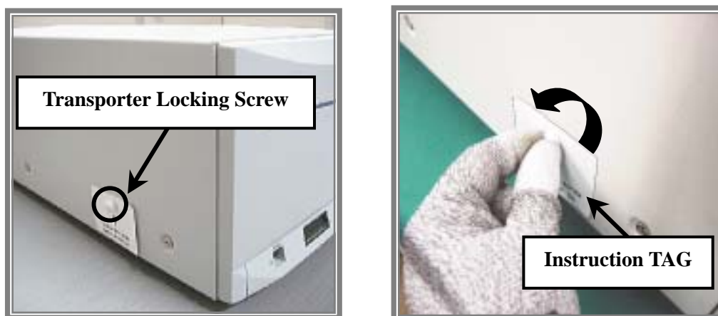
Figure 2-1 Removal of the Transporter Locking Screw and Instruction TAG
