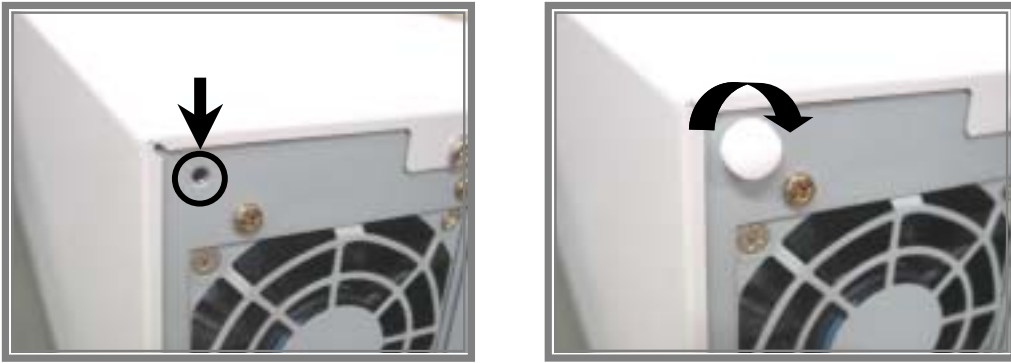
Figure 2-2 Storing the Transporter Locking Screw for later use
