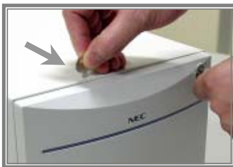
Figure 3-9 Using the Emergency Release Key
