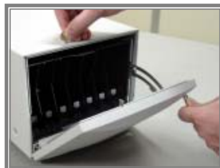
Figure 3-9 Using the Emergency Release Key
