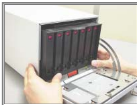
Figure 3-3 Loading the Magazine
