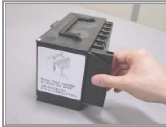
Figure 3-5 Loading the Magazine
